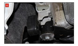
A) Before fitting the Scorpion system, you must rotate the rear mounts by 180° on both sides of the car.
